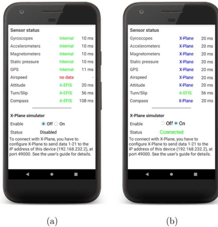
Figure 19: Sensor status screen. (a) A-EFIS with internal sensors, (b) A-EFIS connected to X-Plane flight simulator
