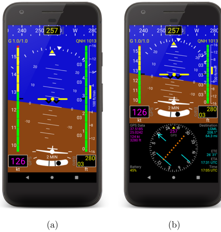
Figure 2: Main EFIS screen in portrait mode. (a) AHRS only layout, (b) AHRS + HSI layout.
