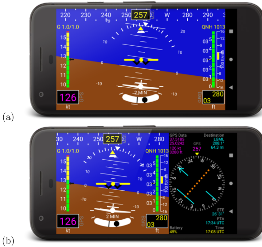
Figure 2: Main EFIS screen in portrait mode. (a) AHRS only layout, (b) AHRS + HSI layout.
