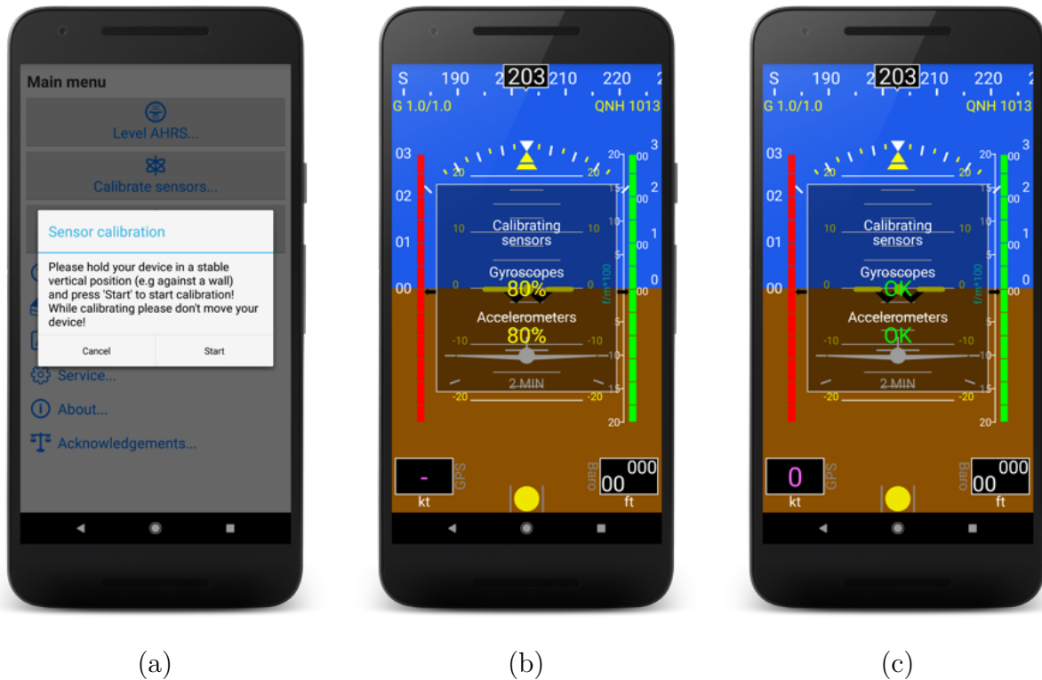
Figure 10: Sensor calibration. (a) Press “Start” to begin sensor calibration. (b) Sensor calibration in progress. (c) Sensor calibration finished.
